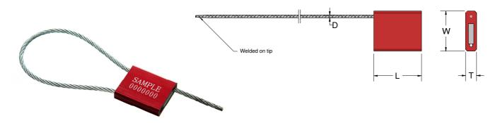
The Acme **CS1 Cable Seal** is available in various cable lengths and diameters to suit all requirements. The lock body is manufactured from die-cast aluminum and the cable from non-preformed galvanized steel. The cable has a welded tip for ease of locking and should the cable be cut it unravels making it impossible to re-lock the seal again without showing obvious signs of tampering. The cable seal require cutters for removal.
