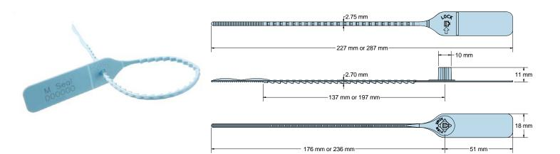
The Acme **M Seal** is a pull tight seal manufactured from Polypropylene material. The locking action is very similar to the tried and tested Minitight but has the contours of the smooth X Seal. The design offers a cost effective solution for applications where strength is not the primary requirement, but is ideal for use as an indicative seal.
