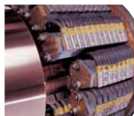
Schunk carbon brushes provide a current transmission of more than 40,000 amperes
